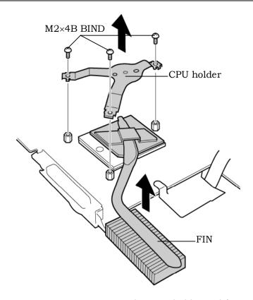
Figure 4-28 Removing the CPU holder and fin
